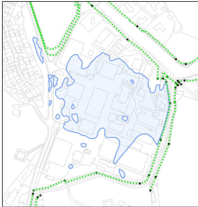
Figure 5: 1 in 200yr surface water flooding, Vector Aerospace (assuming surface water interceptor installed on Main Street)
