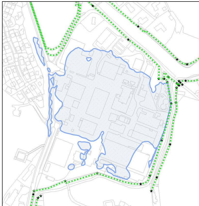
Figure 6: 1 in 200yr surface water flooding, Vector Aerospace (assuming no surface water interceptor on Main Street)
