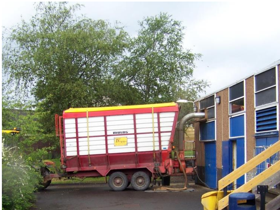
Biomass fuel delivery to Pitlochry High. Fuel store and boiler housed in existing buildings © PKC
