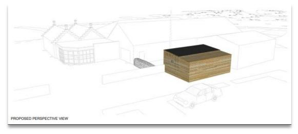
This unit was clad in natural timber, to improve on the temporary look of the building and to appear as a family of visitor infrastructure around the Loch, as the cladding closely matches a recently constructed bird hide on the trail.
