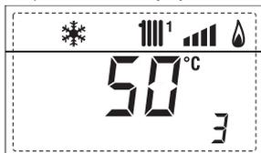
4. Display of auxiliary temperature sensor
