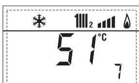
8. Display of ionisation current in  $\mu\text{A}$
