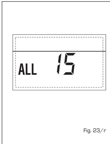
**ATTENTION:** If error "ALL 04" is displayed, the setting of PAR 2 is incorrect. Ensure that PAR2 is set to value 3 (see section 3.3.1).
