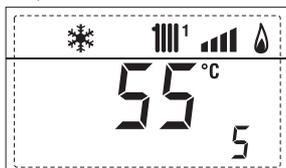
6. Display of heating temperature of first circuit
