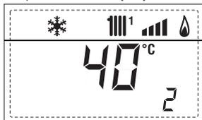
3. Display of D.H.W. temperature sensor (SS)
