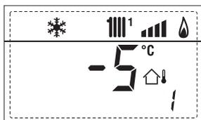
2. Display of heating temperature sensor (SM)
