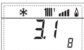
9. Display of fan speed in rpm x 100 (eg 4.800 and 1850 rpm)
