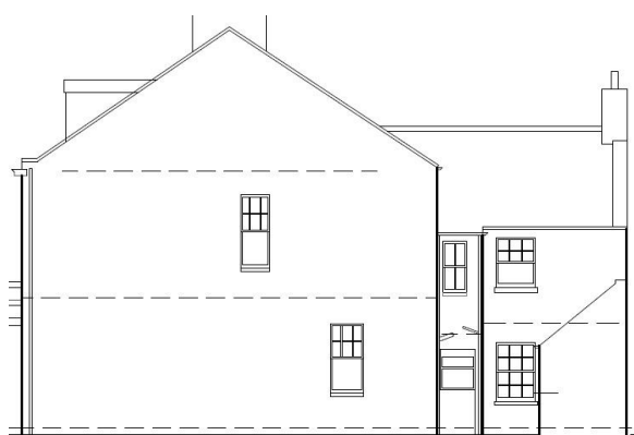
Diagram illustrating the mechanical extract locations and window types for a house: Mechanical extract from bathroom taken through wall Mechanical extract from shower Reduced width window installed, natural stone used to form reveal Mechanical extract from WC taken through wall Mechanical extract from kitchen - taken through Existing window refurbished
