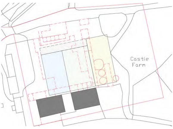
Figure 4 - Demolition Plan (buildings being demolished shown as dashed red)
