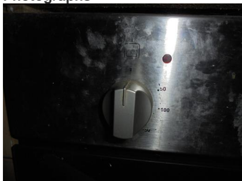
Missing identification function and temperature markers for the oven.
