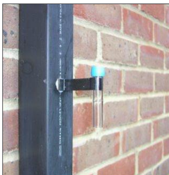
Figure 2.1: Real Time Monitor in Bridgend, Perth (Left), Nitrogen Diffusion Tube (Right)
